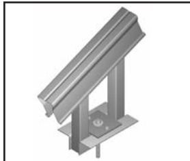
Truss top chord hanger detail
