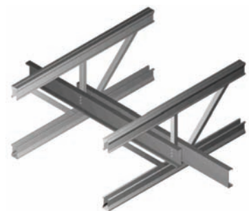
Strongback splice - overlap one truss as shown.
